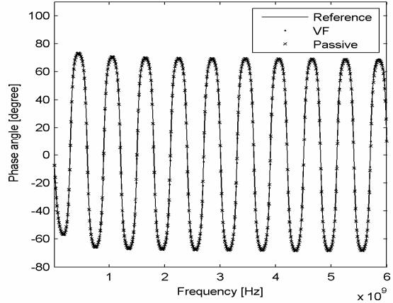
Fig. 2 Phase angle of the reference function  $Z_{II}(f)$  compared to those of identified functions via VF and PFVF algorithms.
