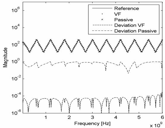
Fig. 1 Magnitude of the reference function  $Z_{II}(f)$  compared to those of identified functions via VF and PFVF algorithms.
