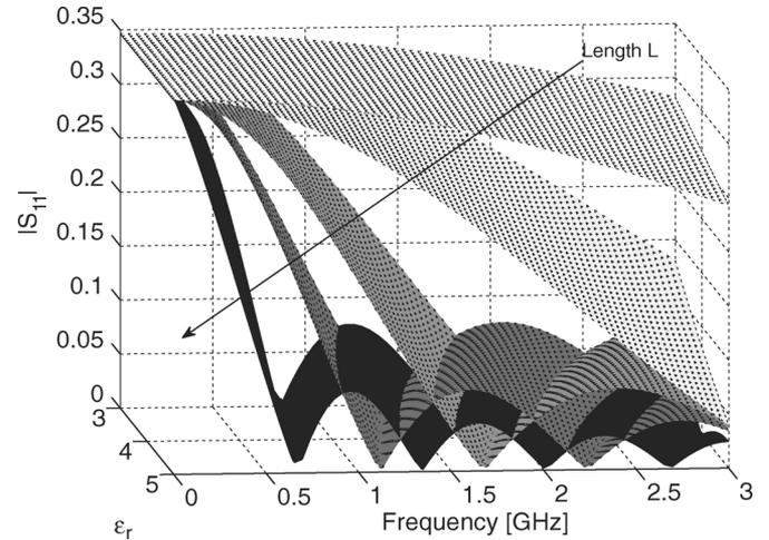
Fig. 12. Reflection coefficient  $S_{11}$  for  $L = 1, 2, 4, 6, 10$  cm.
