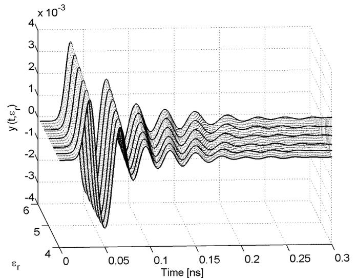
Fig. 8. Bivariate time-domain macromodel of patch antenna.
