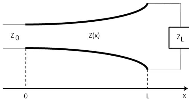
Fig. 10. Exponential tapered microstrip transmission line [27].
