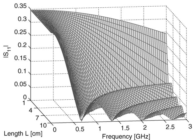
Fig. 11. Reflection coefficient  $S_{11}$  for  $\epsilon_r = 5$ .
