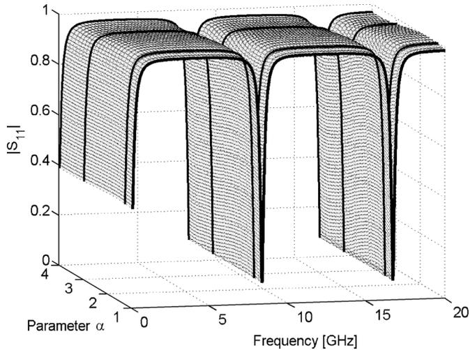
Fig. 1. Magnitude parametric frequency response of interconnect.
