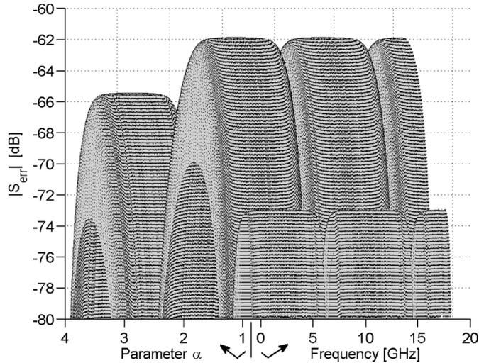
Fig. 5. Absolute error of interconnect introduced by passivity enforcement.
