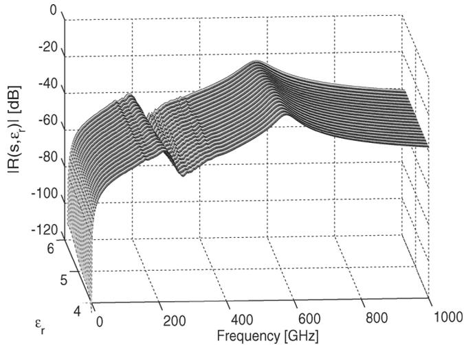
Fig. 9. Bivariate frequency-domain macromodel of patch antenna.
