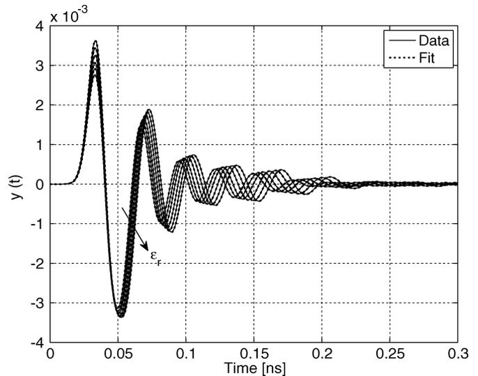
Fig. 7. OVF approximation of six univariate nodes of patch antenna.
