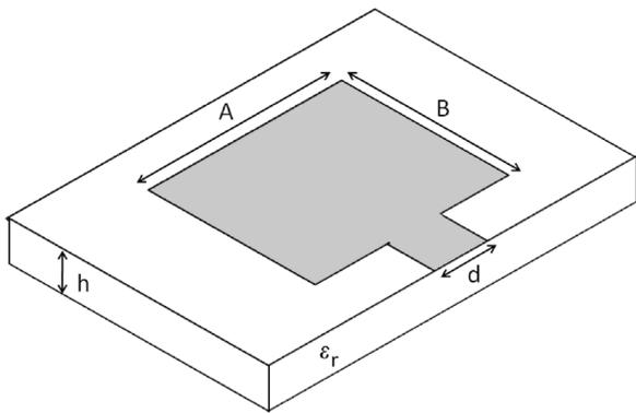
Fig. 6. Rectangular microstrip patch antenna.
