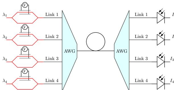
Figure 2. Functional diagram of the WDM system.
