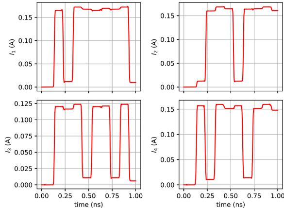
Figure 4. Transient output response of the WDM system simulated in Caphe.
