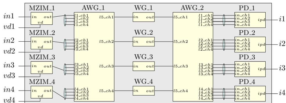
Figure 3. Schematic diagram of the WDM system.
